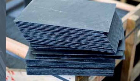
The completed roofing slate. Everyone of them was carefully mined, processed and checked.
